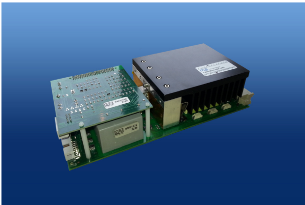
Source-Measure-Unit SMU1022 (200 V, 400 mA, 20 W)
